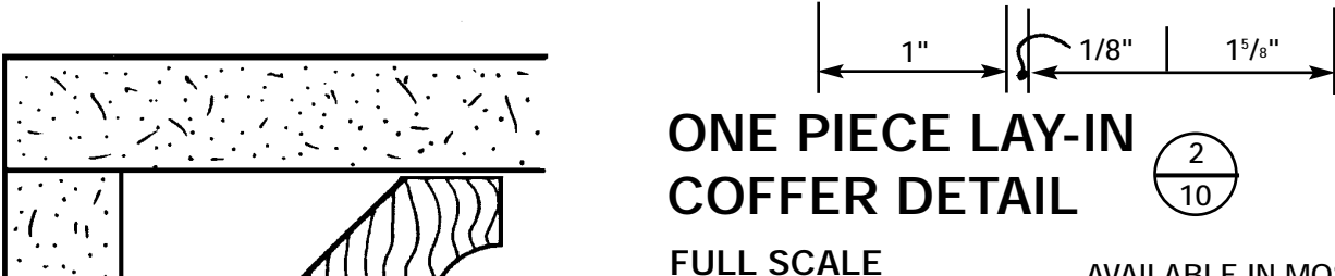
SECTION THRU CROWN MLDG. & COFFER 1 10 FULL SCALE
